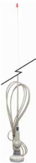
APM01 [White] 27MHz Marine Fibreglass Antenna Overall length: 1400mm Mast length: 1260mm Ground independent (DC) Frequency: 27.880MHz Cable length: 3.6m coaxial Connector: P1259
