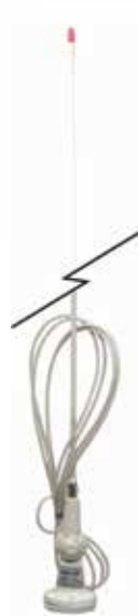
APM03 [White] AM/FM Marine Fibreglass Antenna Overall length: 1150mm Mast length: 1010mm Ground independent (DC) Frequency: AM/FM (receive) Cable length: 3.6m coaxial Connector: P1259
