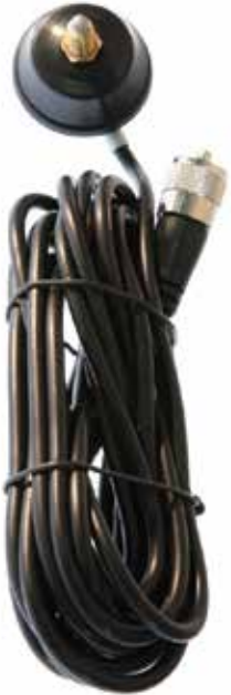
CBBL1 Base and Lead Frequency: 477 MHz UHF 27 MHz AM Length: 5m Cable: RG58 copper shielded coax Connector: PL259
